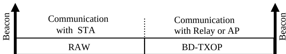
Figure 4.7: Channel access frame for RAP or AP
